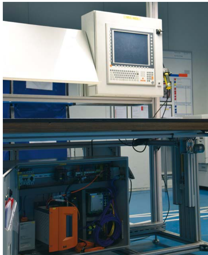
B&R's Automation PCs are installed on 95% of all the lines, sometimes in combination with single-touch or multi-touch Automation Panels.
