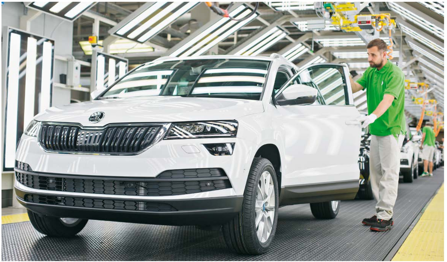
At a speed of 11 meters per minute, one autobody leaves the line every 37 seconds – around the clock, 24-hours a day.
