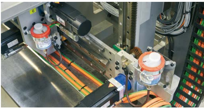
The line features a total of 52 B&R servo motors controlled by ACOPOSmulti drives, six stepper motors controlled by X20 modules and four asynchronous motors controlled by ACOPOSinverters.
