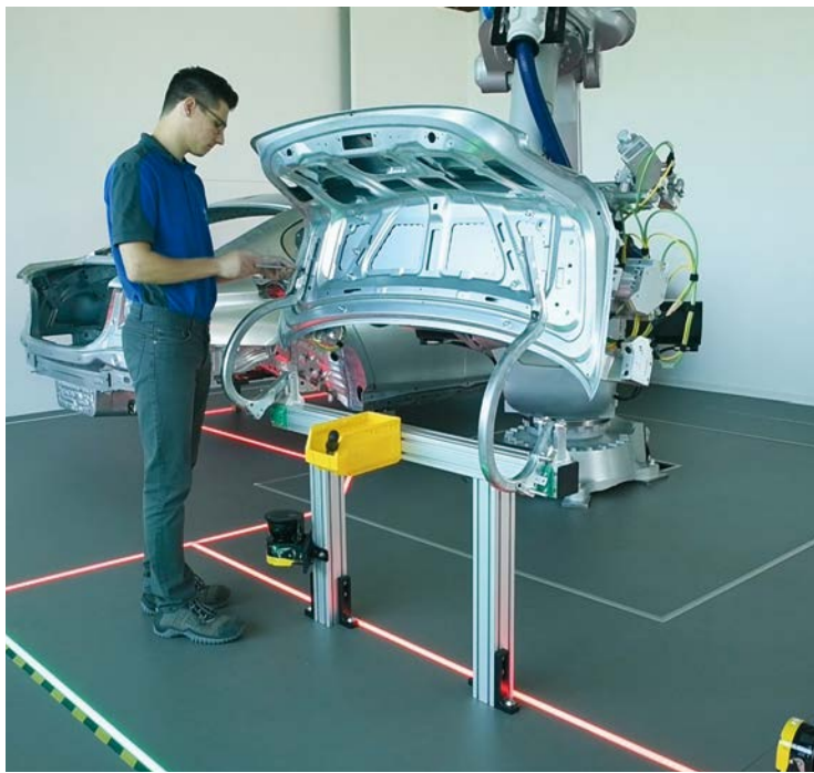
The robot assumes a safe stop state, holding the workpiece in place while the hinges are fastened manually.
