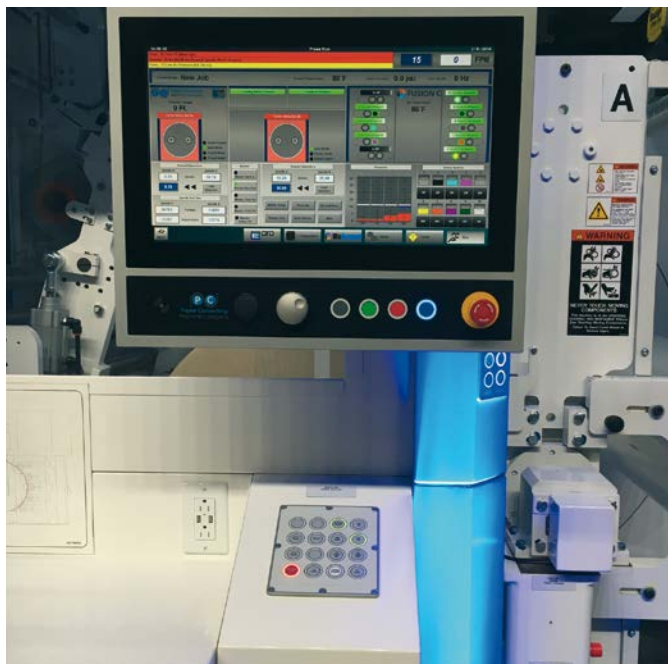
PCMC and B&R co-developed solutions – such as networked illuminated ring keys – which simplify the machine’s control topology by replacing hardwired components such as pushbuttons.
