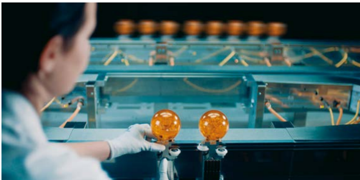
To switch products, the operator simply places the wheels of a new shuttle on the guides of the pit lane, while production continues at full speed on the rest of the track.
