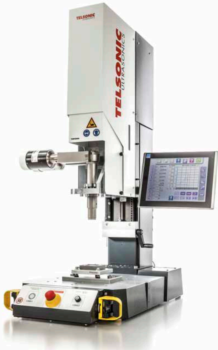
Telsonic's high-precision TPS300 torsional press is designed for large welding objects, delivering a welding force of 3,000 N at 6,500 W of power and a frequency of 20 kHz. The control solution is built around the X20 system from B&R.
