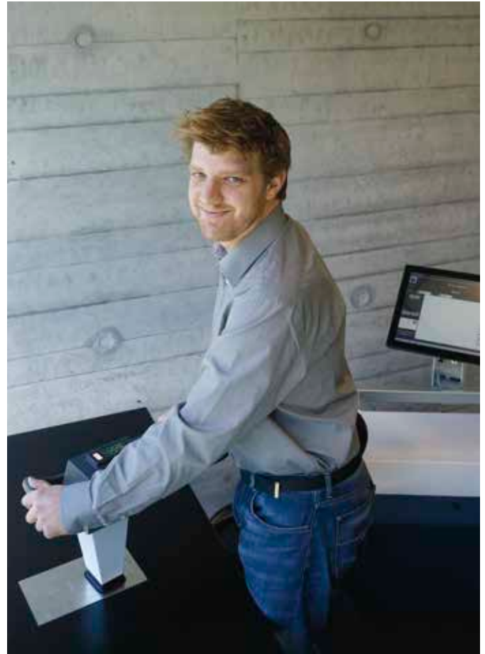
Working without safety glasses: Advanced safety technology such as the SafeLOGIC-X helps the mobile marking laser achieve Class 1 laser protection.
