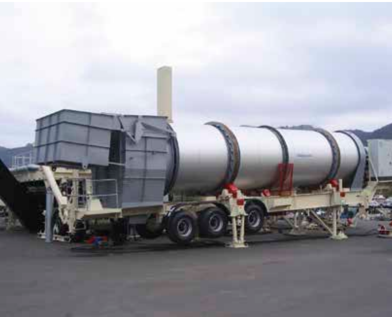
Mobility is a key requirement in hot recycling of damaged pavement. The mobile drum operates with a heated tilting hinge. Hydraulic legs provide precise vertical positioning.
