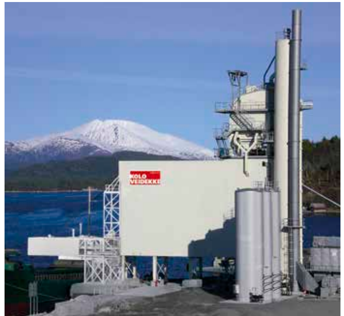
Specialized tank that stores various types of bitumen to meet recipe requirements with greater flexibility.
