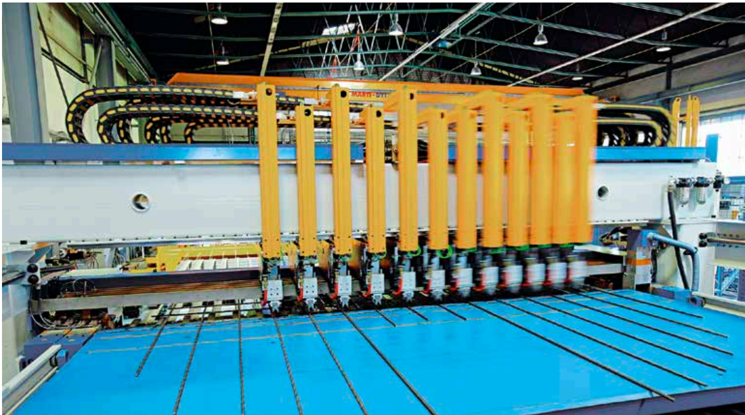
Schlatter's "MG630 Tailor" is an extraordinarily flexible line that produces complex reinforcement mesh in virtually any geometric pattern.
